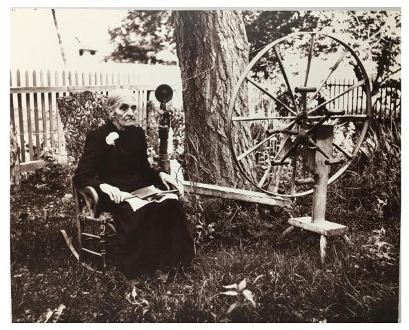
Spinning is the first, and important, part of textile manufacturing. A spinning wheel is used to twist materials, like cotton or wool, and draw them out into thread or yarn that is made into textiles or clothing. Before the spinning wheel was invented in India between 500 and 1000 CE, the spinner would have to do this process by hand. The Great Wheel, one of the earlier types of spinning wheels, is over 5 feet tall. To use it, yarn is tied onto the base of a spindle and connect-
